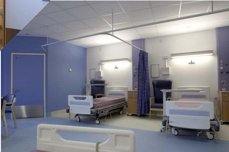
In this example, the en-suite opens directly off the bed area – an alternative arrangement is to have the en-suite in an entrance lobby.
